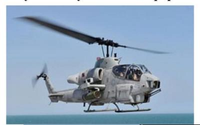
The Bell AH-1 Super Cobra is a twin engine attack helicopter based on the U. S. Army's single engine AH-1-Cobra.
